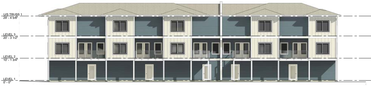
2 B1 EAST ELEVATION (COLOURED) A-202 1/8" = 1'-0"
