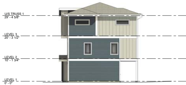
4 B1 SOUTH ELEVATION (COLOURED) A-201 1/8" = 1'-0"
